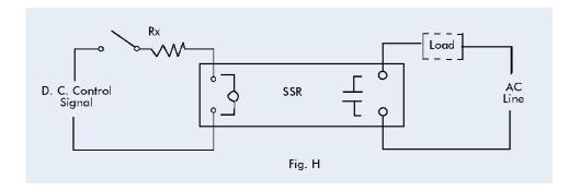
The LOAD can be any one of the numerous types previously discussed. The relay could be an HSSR as well as an SSR.
