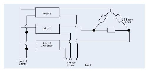
The relay inputs can be supplied in parallel (as shown).
