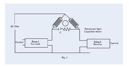
The circuit functions by turning on RELAY 1 or RELAY 2 to drive the motor in the forward or reverse direction. The reversing action is accomplished by changing the electrical location of capacitor C relative to the two motor windings.
