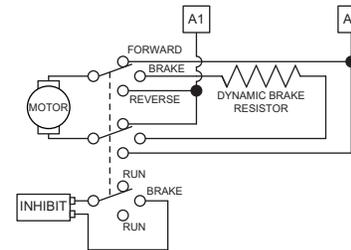
3P3T Relay for Forward/Brake/Reverse
