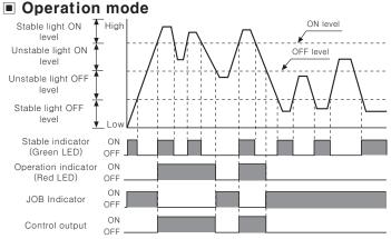
\*The waveform of output. JOB indicator and operation indicator are the state of operation for Light-ON mode, but in case of Dark-ON mode, it is opposite operation against Light ON mode.
